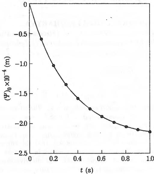
Fig. 1. The mechanical response of piezo-quartz bar time-dependent electrical and thermal excitations
