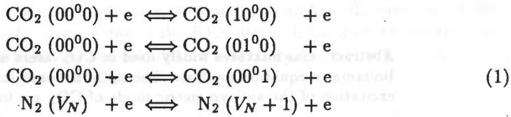
where  $(V_1 V_2^1 V_3)$  notes the respective vibrational modes of CO<sub>2</sub> molecules and  $V_N$  is the quantum number of the N<sub>2</sub> vibrational levels.
