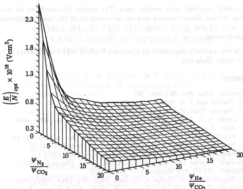
Fig. 1. Optimal  $E/N$  value plotted versus the fractions of  $N_2$  and He molecules in  $CO_2:N_2:He$  mixtures
