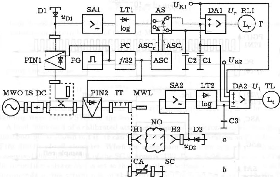
Fig. 1. Block-diagram of the microwave reflectometer (a) circuit for studying the transmissivity of natural objects; (b) the load used for tuning and calibration
