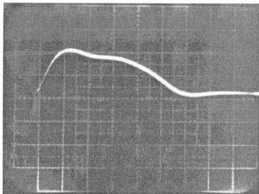
Fig. 3. Typical current pulse shaped using a bopole circuit
