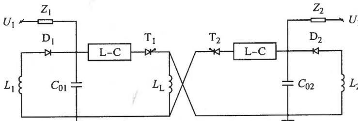
Fig. 4. A six-pole circuit with common inductive load
