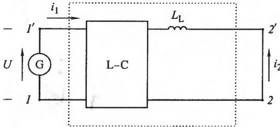
Fig. 1. Schematic representation of a shaping circuit with an inductive load
