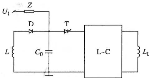
Fig. 2. An example of energy-recuperation shaping circuit with an inductive load
