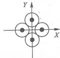
Fig. 5. A double receiving fiber pair permitting measurement of angular misalignments along two orthogonal directions
