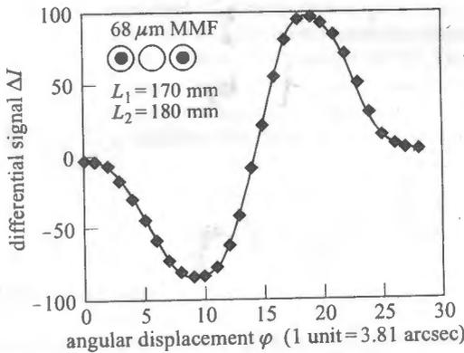
Fig. 4. Differential response of the sensor with a multimode receiving fiber pair and a central fiber
