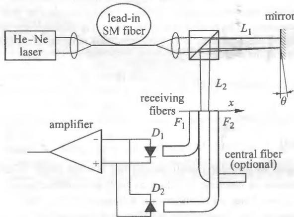
Fig. 1. Schematic representation of the differential angular alignment system
