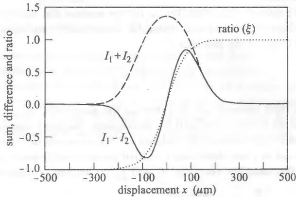
Fig. 2. Difference, sum and ratio of  $I_1$  and  $I_2$  for  $D = 125 \mu\text{m}$  and  $\omega = 100 \mu\text{m}$
