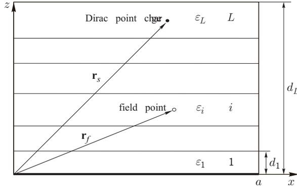
**Fig. 1.** Geometry of a layered structure for multilayer Green's function determination
