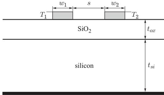
**Fig. 4.** Asymmetric coupled interconnects on lossy silicon substrate
