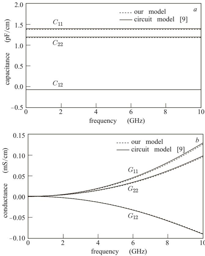
**Fig. 5.** Self and mutual capacitance (a) and self and mutual conductance (b) per unit length of asymmetric coupled interconnects on lossy silicon substrate
