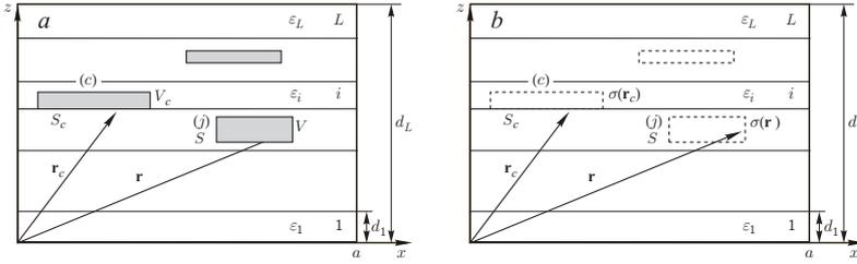
**Fig. 2.** Geometry of a layered structure with (a) embedded conductors, and (b) charge density distribution on the discretized surface of the conductors
