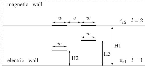
**Fig. 3.** Geometry of the structure from example with four strips  $W/H1 = S/H1 = H2/H1 = 1/3$ ,  $H3/H1 = 2/3$ ,  $\epsilon_{r1} = 5$  and  $\epsilon_{r2} = 1$
