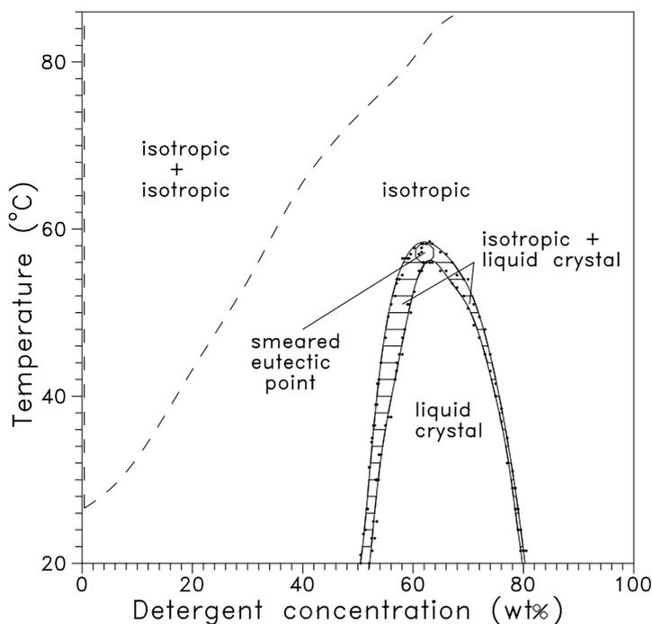
Figure 1. Phase diagram of the Triton X-114 — water binary system for temperatures higher than 20°C.
