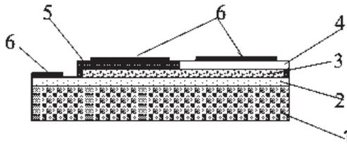
Figure 1. General appearance of an AC HEL display structure: 1 glass substrate; 2 transparent conductive  $\text{SnO}_2\text{:F}$  layer; 3 active layer with a yellow emission; 4 protective vacuum evaporated  $\text{As}_2\text{S}_5$  layer; 5 protective vacuum evaporated  $\text{Ge}_5\text{Sb}_{35}\text{S}_{60}$  layer; 6 Al electrodes.
