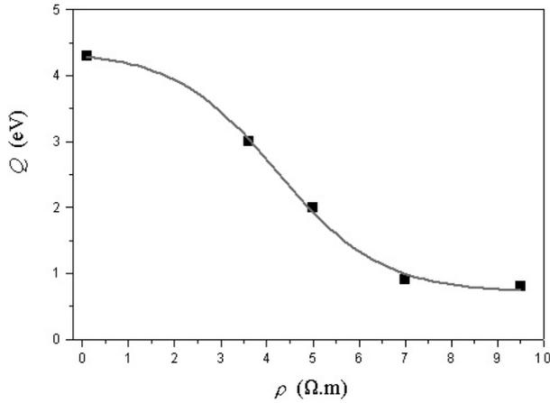
Figure 1. The erasure activation energy  $Q$  of 8-*OBA* versus the specific resistivity  $\rho$  of ITO layer deposited on glass surface.
