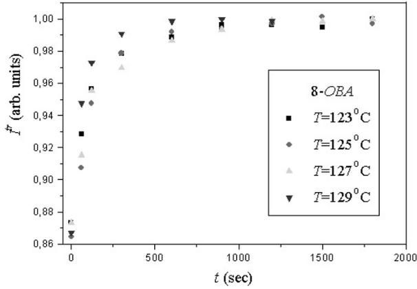
Figure 2. The transmitted light intensity  $I^{tr}$  of 8-OBA versus erasure time  $t_{er}$  at  $t_{rec} = 18 \times 10^2$  sec for different  $T_{er}$ .
