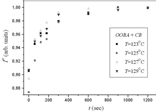
Figure 3. The transmitted light intensity  $I^{tr}$  of 8-*OBA* + *CB* versus erasure time at  $t_{rec} = 18 \times 10^2$  sec for different  $T_{er}$ .
