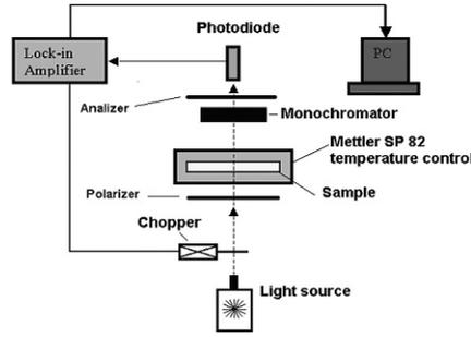
Figure 4. The set-up for spectral – polarization experiment .
