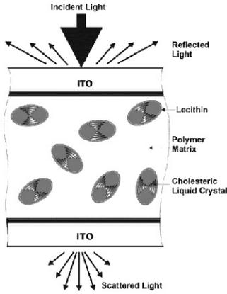
Figure 3. Cross-sectional of PDLC thin film prepared like LC cell.
