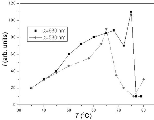
Figure 6. Spectral response of PSLC and PDLC in the active region.
