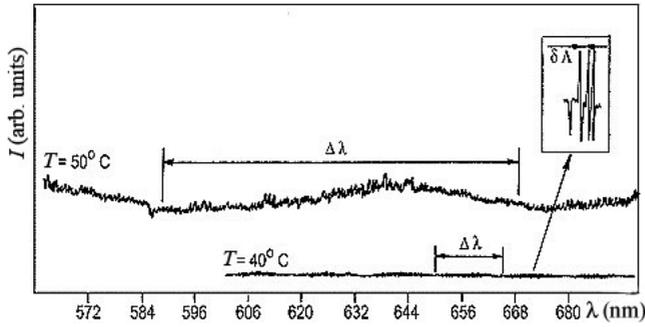
Figure 5. Spectral response of PSLC and PDLC.
