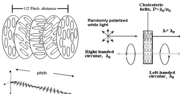
Figure 2. Schematic presentation of the wavelength and pitch of ChLC's.
