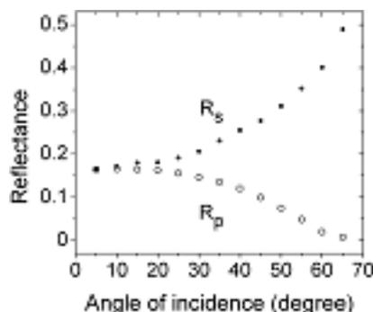
Figure 1: Experimental data for reflectance of  $\text{Si}^+$ -implanted PMMA measured with linearly polarized He-Ne laser beam (wavelength  $\lambda = 632.8$  nm) by two orthogonal polarizations:  $s$  (solid circles) and  $p$  (open circles) versus the incidence angle.
