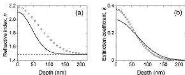
Figure 2: Depth profiles of  $n$  and  $k$  ( $\lambda = 632.8$  nm) derived by: (a) multilayer model and photometry reflectance data (open circles), (b) multiangle-reflection ellipsometrical measurements of  $\text{Si}^+$ -implanted PMMA. The dashed line indicates the refractive index of non-implanted PMMA (in our case 1.490 determined by ellipsometric measurement at  $\lambda = 632.8$  nm).
