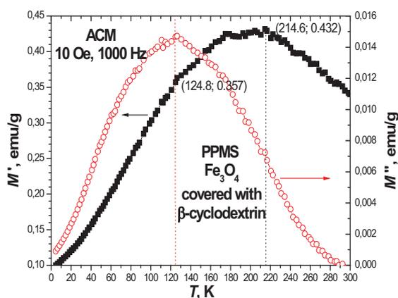
Figure 6. A.c. magnetization of shielded magnetite.
