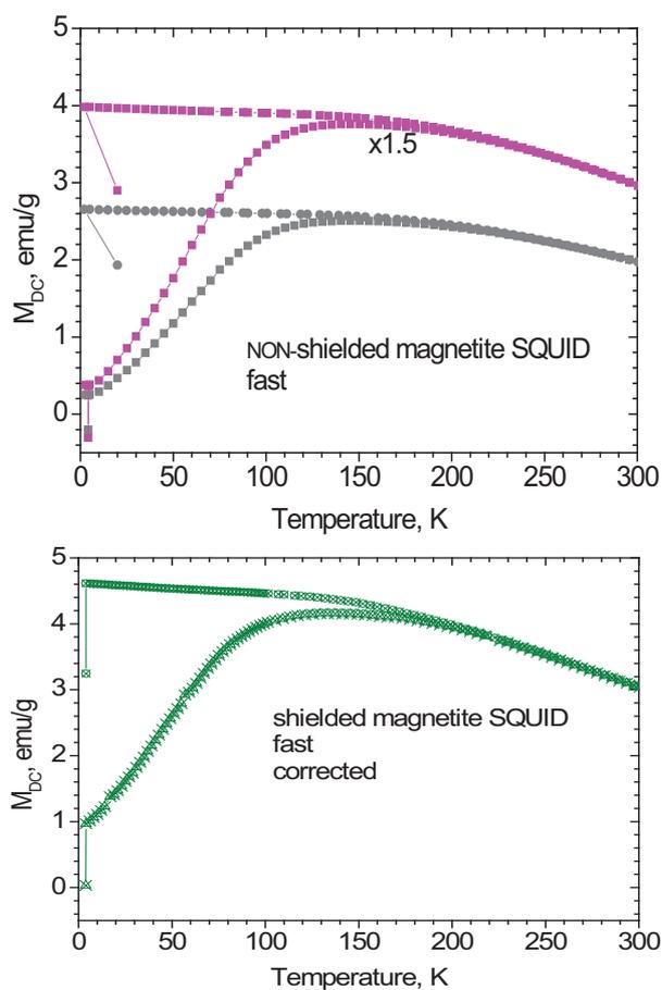
Figure 5. D.c. magnetization vs. temperature for unshielded and shielded nanostructured magnetite.
