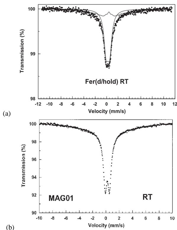
Figure 3. Mössbauer spectra at room temperature of: (a) hybrid particles with magnetic core size  $10 \pm 2$  nm [9] and (b) nanostructured magnetite with grain size  $10 \pm 2$  nm, [9].
