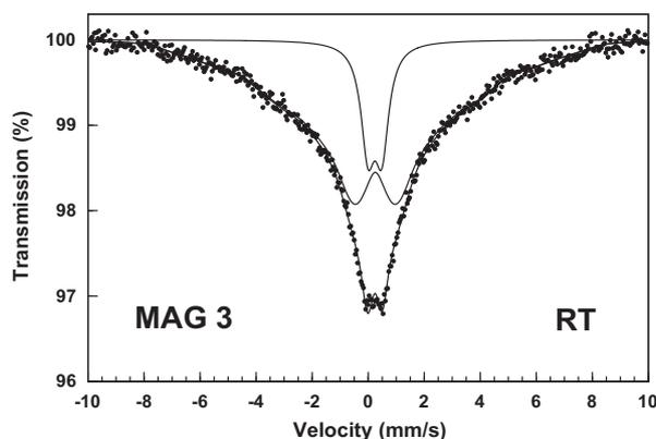
Figure 2. RT Mössbauer spectrum of a sample with organic shield.
