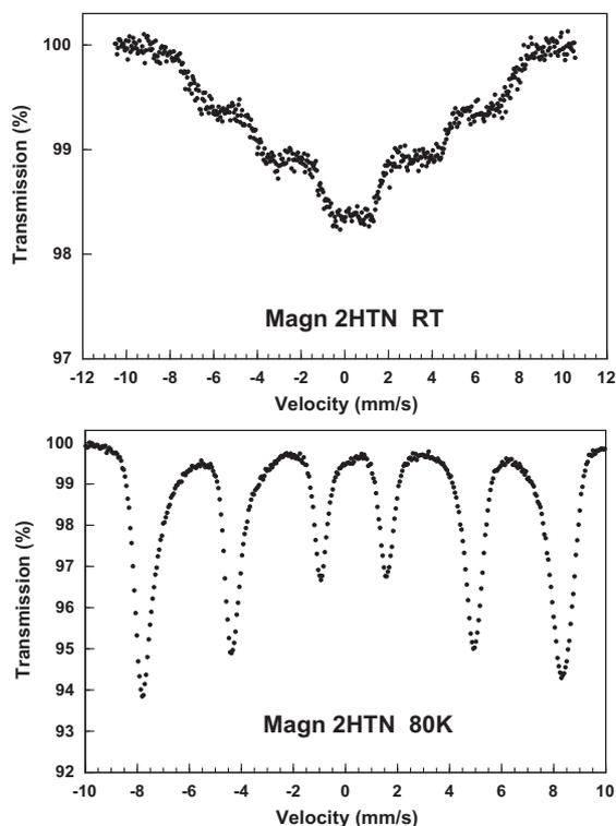
Figure 1. Mössbauer spectra (RT and 80 K) of magnetite particles prepared in nitrogen ambient.
