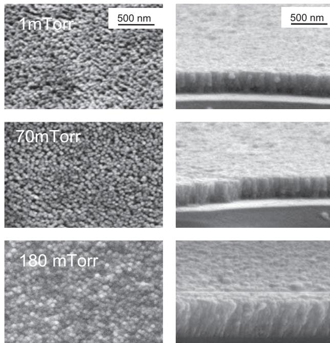
Figure 1. Top- and cross sectional- view SEM images of ZnO layers grown at the indicated partial oxygen pressure  $P_{O_2}$ .
