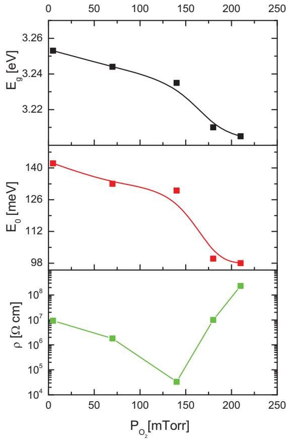
Figure 3. The optical energy gap  $E_g$ , Urbach energy  $E_U$  and the resistivity  $\rho$  of 100 nm thick ZnO layers in dependence of the partial oxygen pressure  $P_{O_2}$ .
