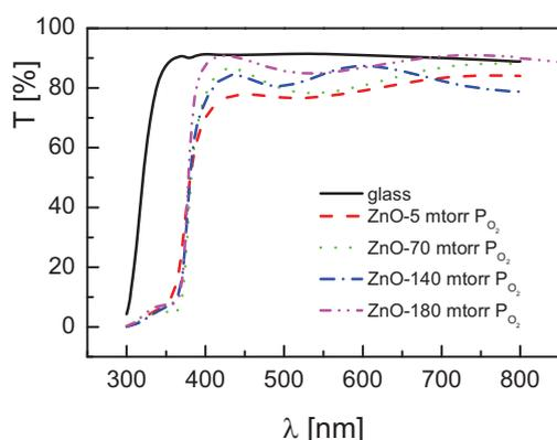
Figure 2. Optical transmittance spectra of glass substrate and 100 nm thick ZnO layers deposited at different oxygen partial pressure  $P_{O_2}$ .
