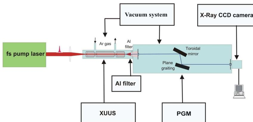
Figure 1. Experimental set-up for phase-matched EUV high-harmonics generation in a capillary waveguide. Fs pump laser – Ti:Sapphire mode-locked femtosecond system (47 fs/1 kHz/3.4 mJ/800 nm). The vacuum system ensures volume evacuation down to  $p \sim 10^{-5}$  mbar. X-Ray CCD camera – Newton DO920-BN-9HC,  $1024 \times 255$  pixels., (Andor Technology). XUUS – eXtreme Ultraviolet Ultrafast Source (KMLabs Inc.). PGM – plane grating vacuum monochromator with 1 m focal length (Horiba Scientific).
