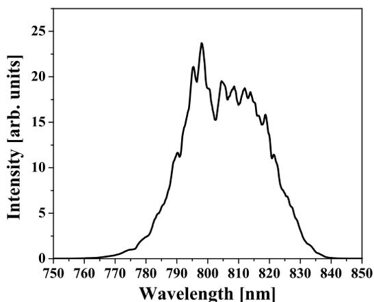
Figure 2. Spectral distribution of the femtosecond pump radiation.
