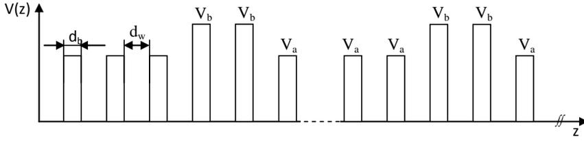
Figure 1. Schematic view of the conduction band-edge profile of the DBSL.
