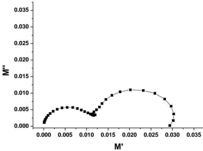
Figure 4. Complex modulus spectrum.
