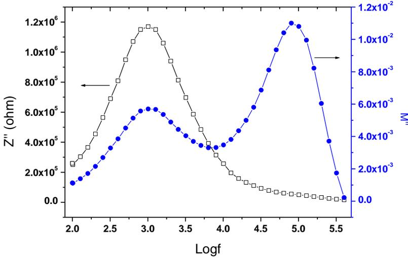
Figure 3. Plots of  $Z''$  versus  $\log f$  and  $M''$  versus  $\log f$ .
