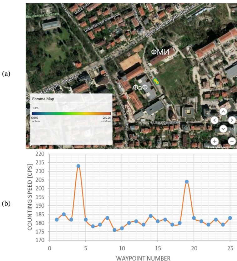
Figure 3. Initial determining of the contamination distribution: (a) using Microsoft 3D Map; and (b) a simple Excel graph.
