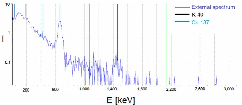
Figure 5. Spectrum integrated for 1 minute hanging over the most significant contamination spot. The SMI software recognizes presence of NORM and Cs-137.
