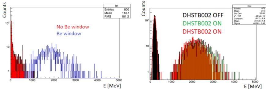
Figure 4. The total energy distribution in the ECAL from the MC of the experiment, with and without the Beryllium window (on the left) compared to the total energy distribution of the collected data (on the right; DHSTB002 is the last dipole of the transfer line before the target) [14].
