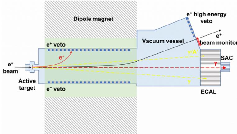
Figure 2. Scheme of the PADME Detector System.
