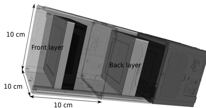
Figure 1. Prototype of a nanosatellite with Compton camera designed in our group and placed inside 3 units CubeSat modules, designed by NASA [6]. Each detector consists of monolithic scintillation crystal coupled to a multi-pixel photomultiplier [7].
