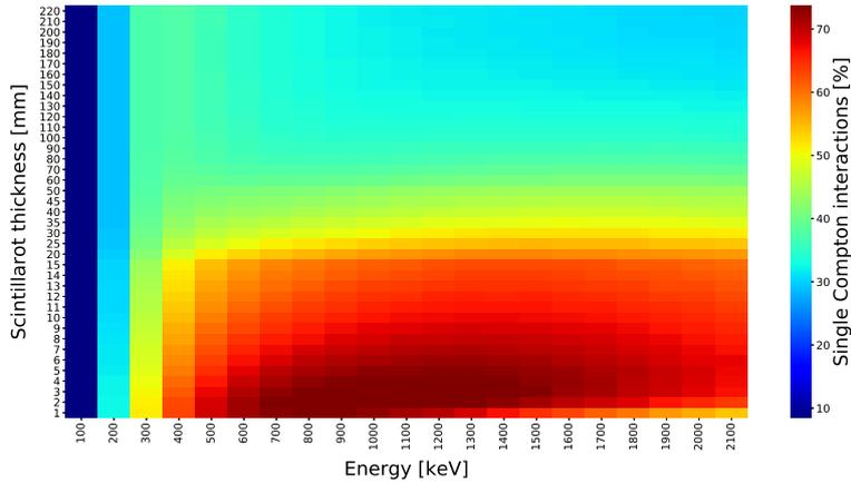
Figure 3. First Compton interaction events for different gamma rays energies and  $\text{CeBr}_3$  scintillation thicknesses.
