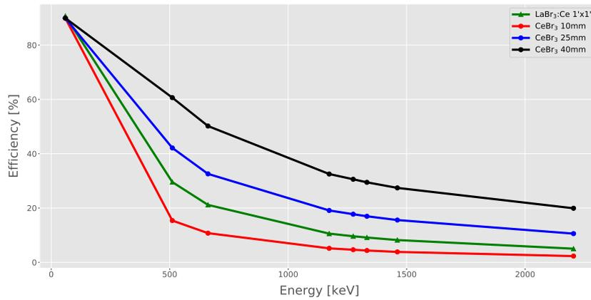
Figure 4. Scintillators efficiency for different gamma rays energies.
