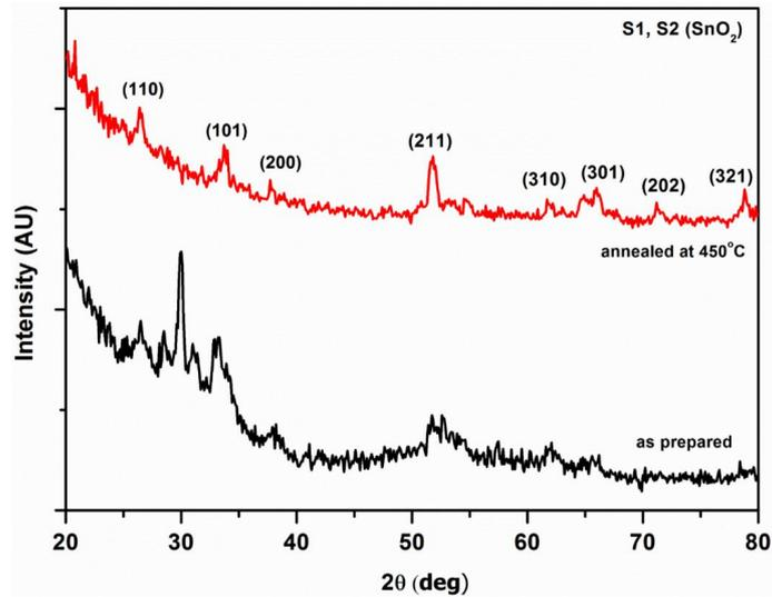
Figure 1. XRD pattern of as prepared and annealed samples with 2M KOH.
