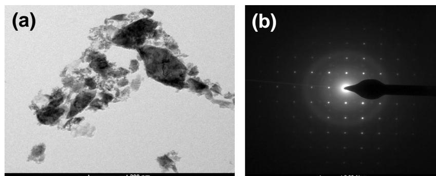
Figure 4. (a) Low magnification bright field image; and (b) SAED pattern of as synthesized SnO (S3) nanostructure.
