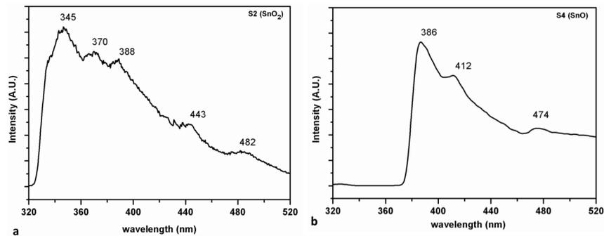
Figure 6. Photoluminescence spectra (excitation wavelength: 320 nm) for: (a) annealed S2; and (b) S4 samples.
