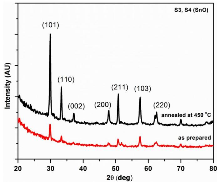
Figure 2. (a) XRD pattern of as prepared and annealed samples with 4M KOH.
