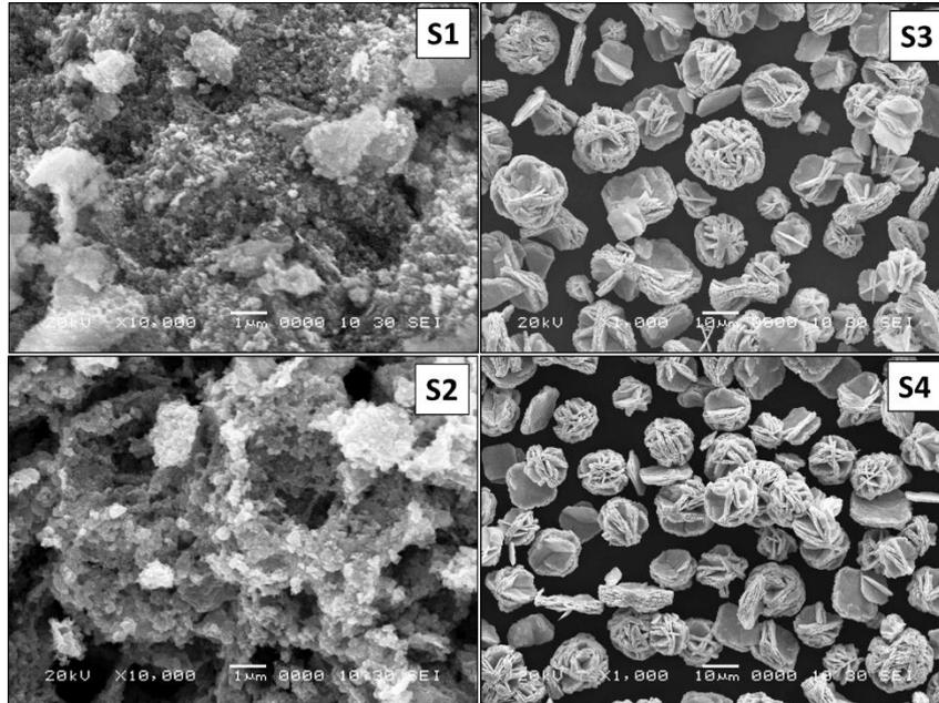
Figure 3. SEM micrographs for as-synthesized SnO<sub>2</sub> (S1) & SnO (S3) and annealed SnO<sub>2</sub> (S2) & SnO (S4) nanostructures.
