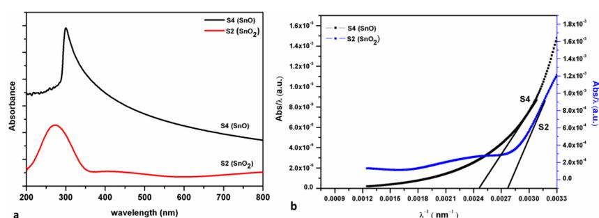
Figure 5. (a) Optical absorption spectra; and (b) band gap energy calculation of annealed samples (S2 and S4).
