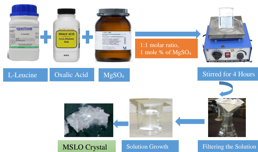
Figure 1. Flow diagram for crystal growth process.
