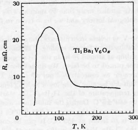
Fig. 2. Resistivity temperature dependence of Tl-Ba-V-O
