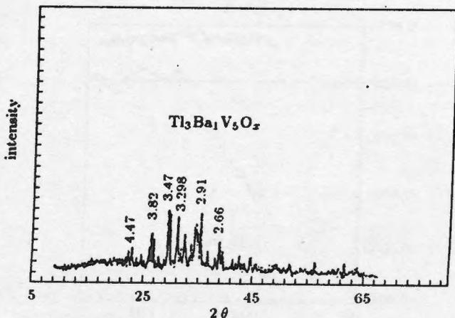
Fig. 1. X-ray powder diffraction spectrum of the 135 phase of Ba-Tl-V-O
