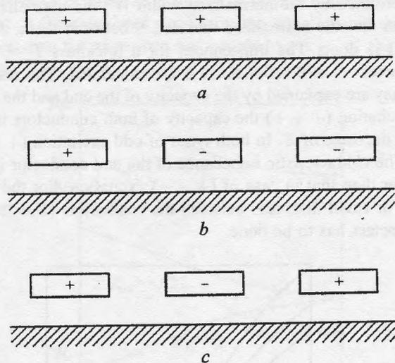
Fig. 2. Three kinds of excitation of three conductor strip line (a) even - (+ + +); (b) odd - (+ - -); (c) odd - (+ - +)
