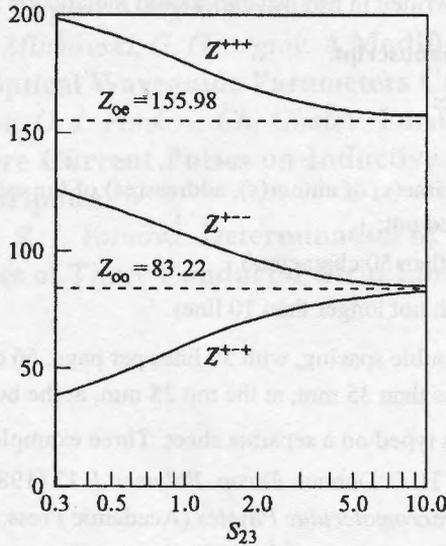
Fig. 5. The influence of distance  $S_{23}$  on the characteristic impedance  $Z_2$
