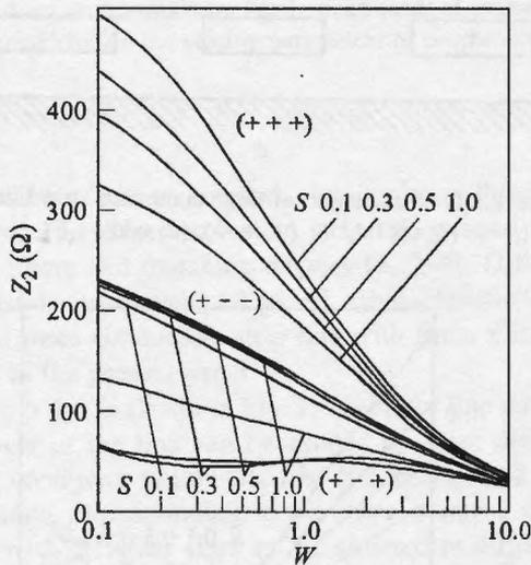
Fig. 4. Characteristic impedance of the middle conductor  $Z_2$
