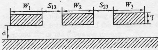
Fig. 1. Cross section of three conductor strip line
