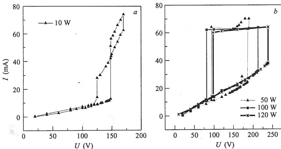
Fig. 4. The dependence of the probe current on the voltage,  $I = I(U)$ , at different RF powers
