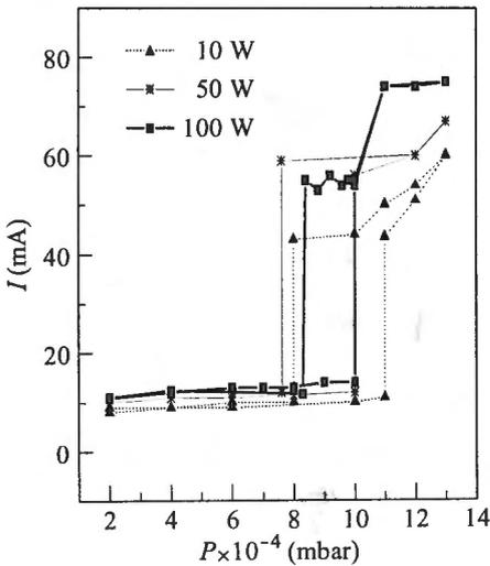
Fig. 5. The dependence of the probe current on the chamber pressure,  $I = I(p)$ , at different powers ( $p = 4 \times 10^{-4}$  mbar)
