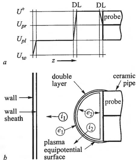
Fig. 3. Qualitative drawing of the potential distribution (a) and double layer on the probe in ICP (b)
