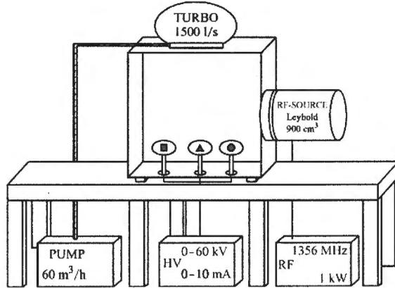
**Fig. 1.** Scheme of the PIII experiment at Frankfurt University. A Leybold ion RF source is mounted to the target chamber and coupled to a 13.56 MHz RF generator (details of the source are presented in [2]). During plasma measurement the targets are put away
