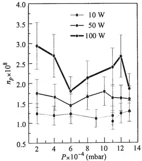
Fig. 6. The increasing of the plasma density with RF power ( $U = 120$  V)
