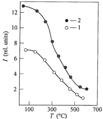
Fig. 4. Temperature dependence of magnetization of rapidly solidified Al-1 wt. % Zn alloy (1) as cast; (2) after implantation with 60 keV Fe ions, dose  $8 \times 10^{17} \text{ cm}^{-2}$
