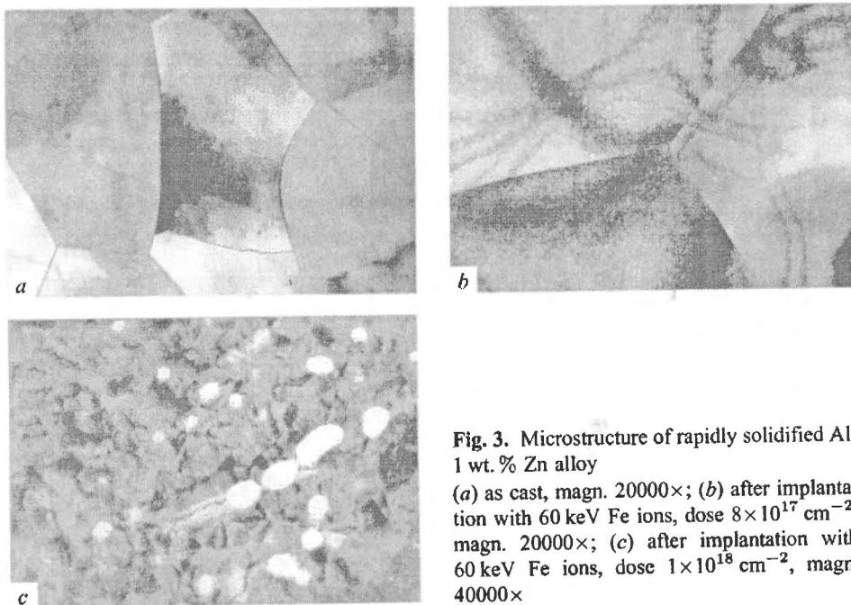
**Fig. 3.** Microstructure of rapidly solidified Al-1 wt. % Zn alloy
