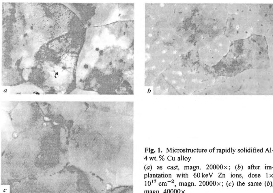
Fig. 1. Microstructure of rapidly solidified Al-4 wt. % Cu alloy
