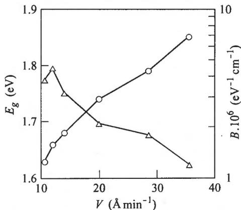
Fig. 1. Deposition rate dependence of the optical band gap  $E_g$  (circles) and constant  $B$  (triangles).  $T_s = 250^\circ\text{C}$
