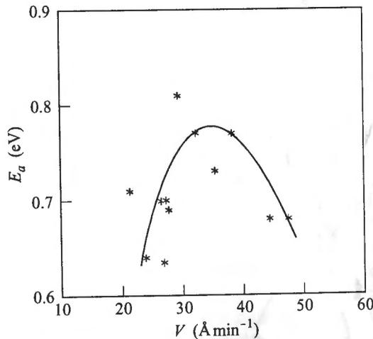
Fig. 5. Deposition rate dependence of the activation energy
