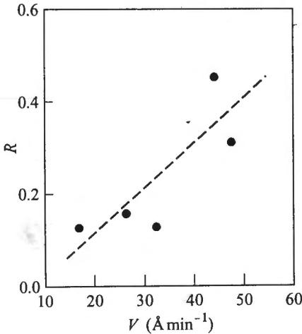
Fig. 3. Dependence of the parameter of microstructure on the deposition rate
