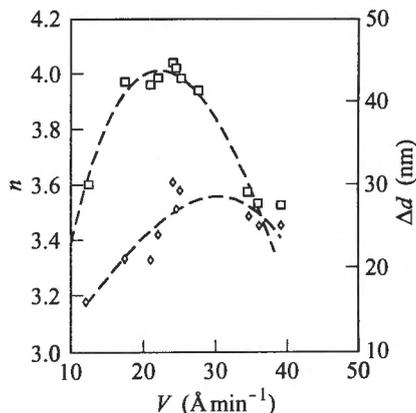
Fig. 2. Dependence of the refractive index  $n$  (squares) and inhomogeneity parameter  $\Delta d$  (diamonds) on the deposition rate
