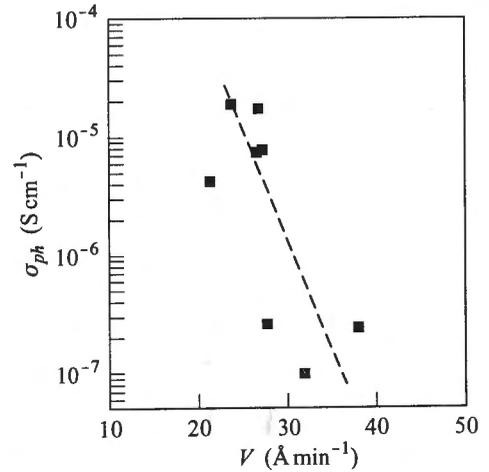
Fig. 4. Deposition rate dependence of the photoconductivity
