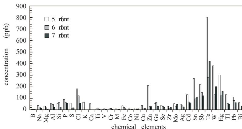
**Fig. 1.** Concentration of residual impurities in the ingot fronts
