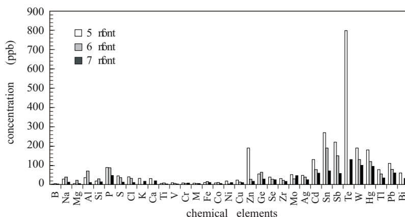
**Fig. 2.** Concentration of residual impurities in the ingot ends
