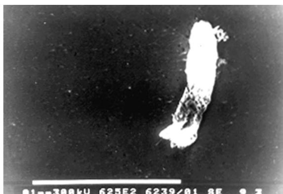
**Fig. 3.** Electron-microscopic research of micro-inclusions in InAs
