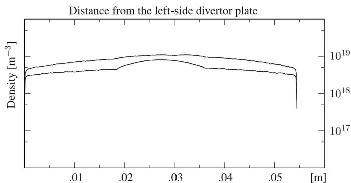
Figure 4. Plasma density profile assuming a neutral density distribution shown in Figure 3a.
