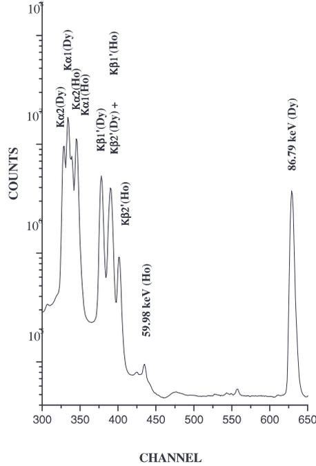
Figure 1. The fragment  $\gamma$ -spectrum from the decay  $^{160}\text{Er} \rightarrow ^{160m,g}\text{Ho} \rightarrow ^{160}\text{Dy}$  (d36 mm  $\times$  13 mm HPGe-detector).
