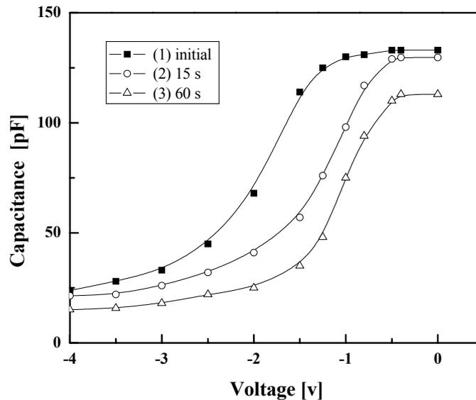
Figure 1. Typical  $C/V$  curves obtained on initial (curve 1) and electron irradiated Si–SiO<sub>2</sub> structures for 15 and 60 s (curves 2 and 3), respectively.
