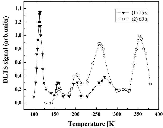
Figure 2. Typical DLTS spectra of the electron irradiated MOS samples after 15 s (curve 1) and 60 s irradiation (curve 2).
