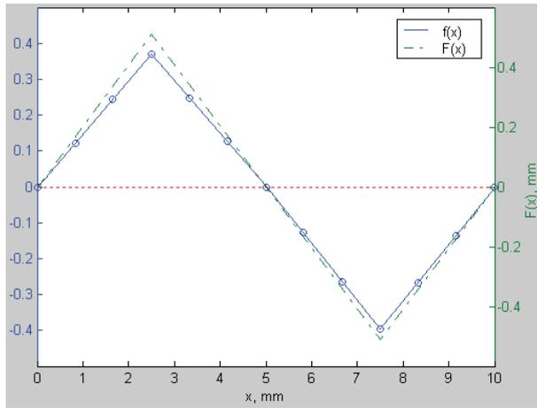
Figure 7. The reconstructed surface profile of the studied object with 80 registered values of the amplitude field and  $\lambda = 1.3636$  mm –  $f(x)$ ; the same profile theoretically calculated with 80 harmonics in the Fourier series –  $F(x)$ .
