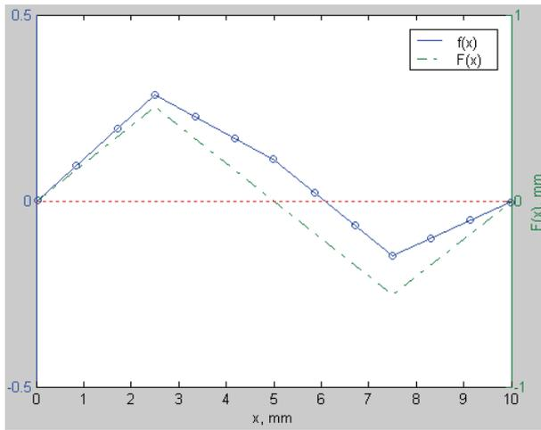
Figure 5. The reconstructed surface profile of the studied object with 45 registered values of the amplitude field and  $\lambda = 0.6818$  mm –  $f(x)$ ; the same profile theoretically calculated with 45 harmonics in the Fourier series –  $F(x)$ .
