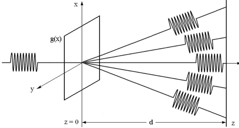
Figure 2. Separation of the harmonic components by the delays.
