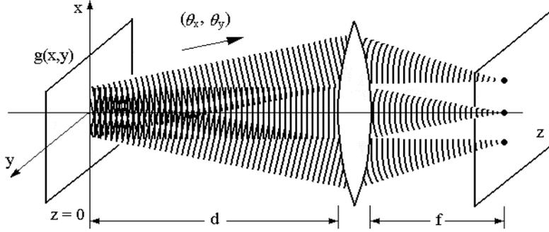
Figure 1. The Fourier transformation of the input wave in the far field.
