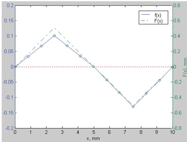
Figure 6. The reconstructed surface profile of the studied object with 40 registered values of the amplitude field and  $\lambda = 1.3636$  mm –  $f(x)$ ; the same profile theoretically calculated with 40 harmonics in the Fourier series –  $F(x)$ .
