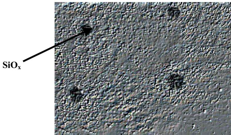
Figure 2. Topography of the silicon substrate etched at 2 kW and 10 mtorr (50 $\times$ ).
