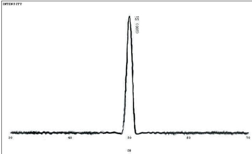
Figure 6. X-ray diffraction pattern for the sample processed at 750 W and 15 mtorr.
