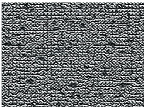
Figure 4. Topography of the silicon substrate etched at 1.2 kW and 15 mtorr ( $50\times$ ).
