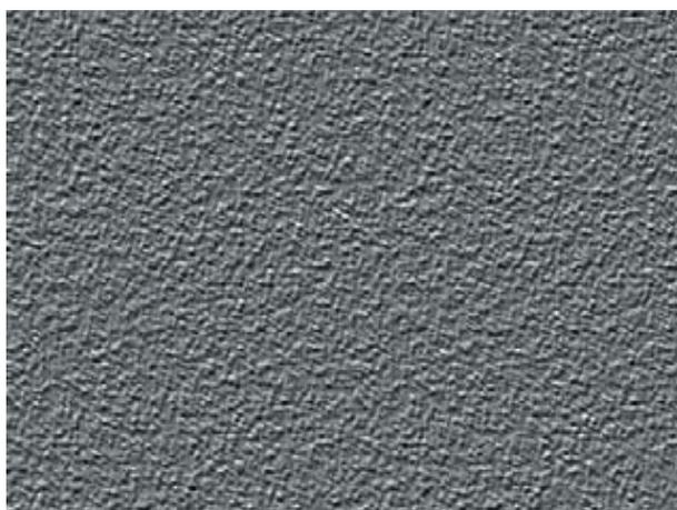
Figure 1. Topography of the silicon substrate processed at 150 W and 10 mtorr (50 $\times$ ).
