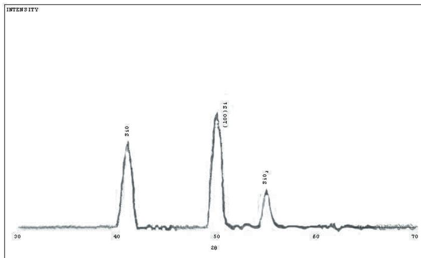
Figure 3. X-ray diffraction pattern for the sample processed at 2 kW and 10 mtorr.
