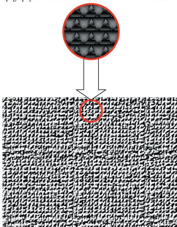
Figure 5. Topography of the silicon substrate etched at 750 W and 15 mtorr ( $50\times$ ).
