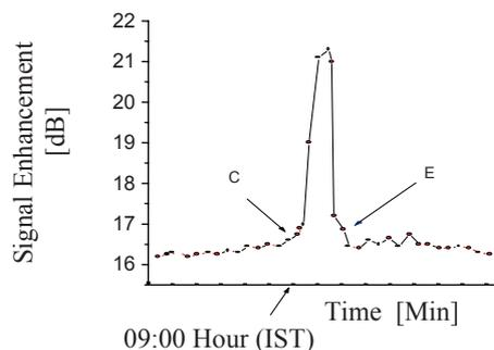
Figure 2. Typical enhancement in signal strength due to solar flare.
