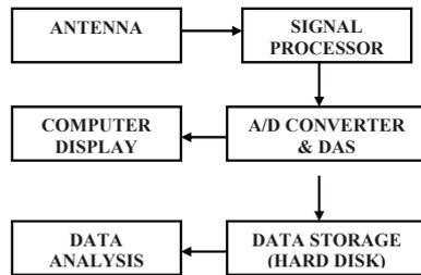
Figure 1. Block diagram of VLF/LF recording system.
