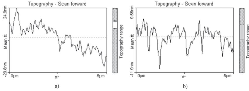
Figure 1. Topography of the surface roughness of: a) s. 127 and b) s. 147, studied by AFM (easyScan2 AFM, Nanosurf, CH)
