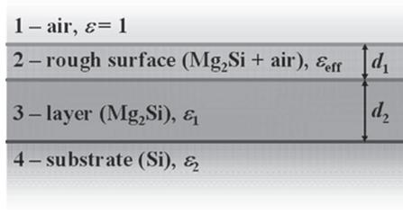
Figure 2. A scheme of the four layer structure used for calculation of the phonon-polariton dispersion relations.
