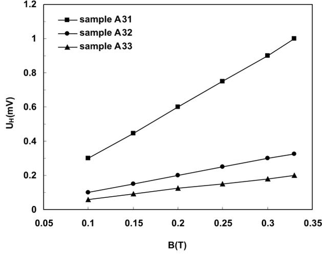
Figure 3. Hall voltage vs. the magnetic induction: sample A31 ( $d = 0.19 \mu\text{m}$ ), sample A32 ( $d = 0.46 \mu\text{m}$ ), sample A33 ( $d = 0.62 \mu\text{m}$ ),  $T_S = 523 \text{ K}$  and  $I = 12.5 \text{ mA}$ .
