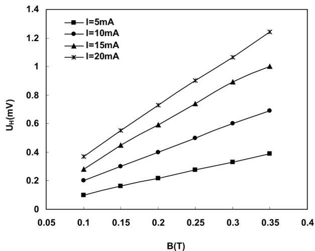
Figure 1. Hall voltage vs. the magnetic induction for sample A21,  $d = 0.22 \mu\text{m}$  and  $T_S = 473 \text{ K}$ .
