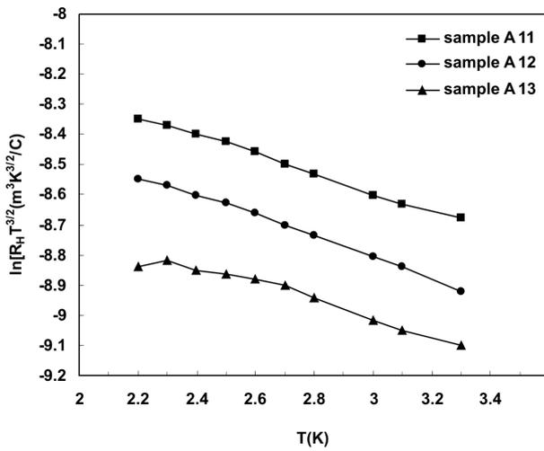
Figure 6. Temperature dependence of the Hall coefficient for films with various thickness: sample A11 ( $d = 0.17 \mu\text{m}$ ), sample A12 ( $d = 0.39 \mu\text{m}$ ), sample A13 ( $d = 0.57 \mu\text{m}$ ),  $T_S = 293 \text{ K}$  and  $B = 0.22 \text{ T}$ .
