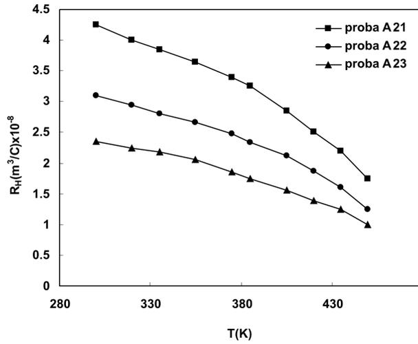
Figure 5. Temperature dependence of the Hall coefficient for films with various thickness: sample A21 ( $d = 0.22 \mu\text{m}$ ), sample A22 ( $d = 0.51 \mu\text{m}$ ), sample A23 ( $d = 0.68 \mu\text{m}$ ),  $T_S = 473 \text{ K}$  and  $B = 0.22 \text{ T}$ .
