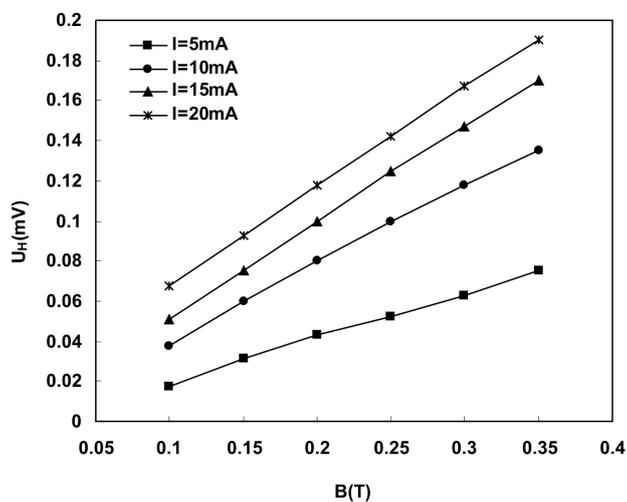
Figure 2. Hall voltage vs. the magnetic induction for sample A23,  $d = 0.68 \mu\text{m}$  and  $T_S = 473 \text{ K}$ .
