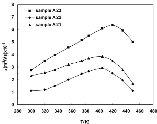
Figure 7. Temperature dependence of the Hall mobility for films with various thickness: sample A23 ( $d = 0.68 \mu\text{m}$ ), sample A22 ( $d = 0.51 \mu\text{m}$ ), sample A21 ( $d = 0.22 \mu\text{m}$ ),  $T_S = 473 \text{ K}$ .
