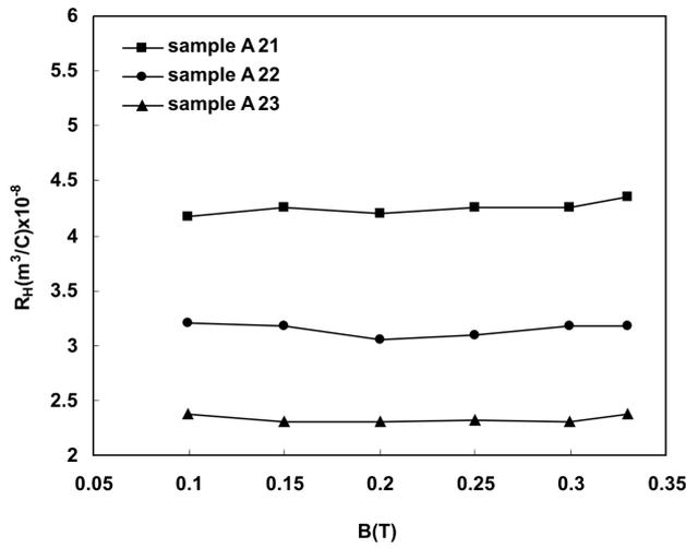
Figure 4. Hall coefficient vs. the magnetic induction: sample A21 ( $d = 0.22 \mu\text{m}$ ), sample A22 ( $d = 0.51 \mu\text{m}$ ), sample A23 ( $d = 0.68 \mu\text{m}$ ),  $T_S = 523 \text{ K}$  and  $I = 12.5 \text{ mA}$ .
