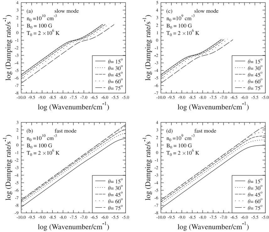
Figure 1. Variation of damping rate as a function of wavenumber for: (a) slow-mode wave and (b) fast-mode wave. Values of parameters are written there.
