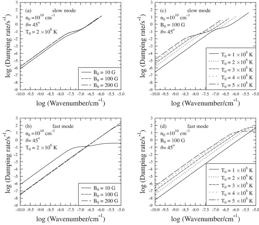
Figure 4. Variation of damping rate as a function of wavenumber for: (a) slow-mode wave and (b) fast-mode wave. Values of parameters are written there.
