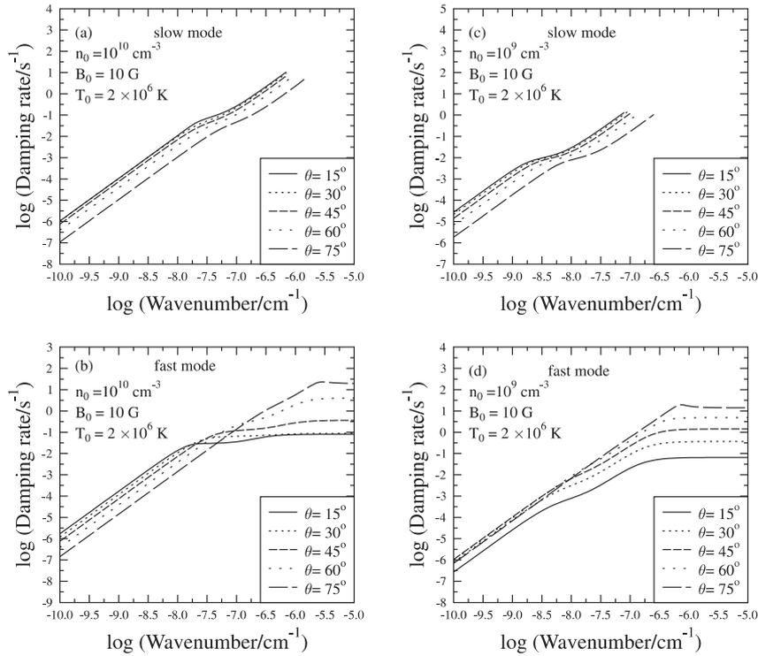
Figure 2. Variation of damping rate as a function of wavenumber for: (a) slow-mode wave and (b) fast-mode wave. Values of parameters are written there.
