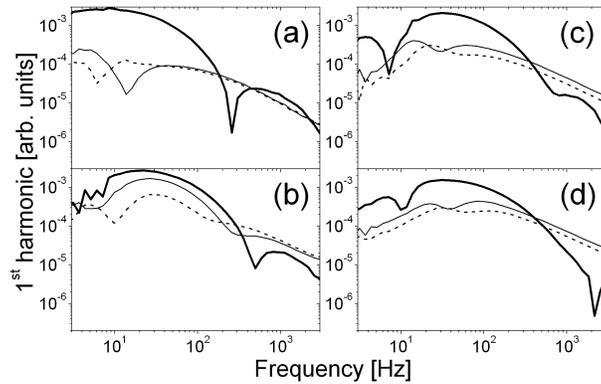
Figure 3. Flexoelectro-optical response of the examined LC-polymer composite layer in twisted cell. The 1st harmonic spectra are plotted for various values of the applied voltage: 3.6 V (dashed line); 4.8 V (thin line); 9.6 V (bold line). The temperature of the sample: 22°C (a); 30°C (b); 35°C (c); 40°C (d).
