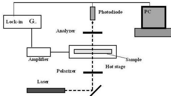
Figure 1. Schematic of the experimental set-up used in this work.
