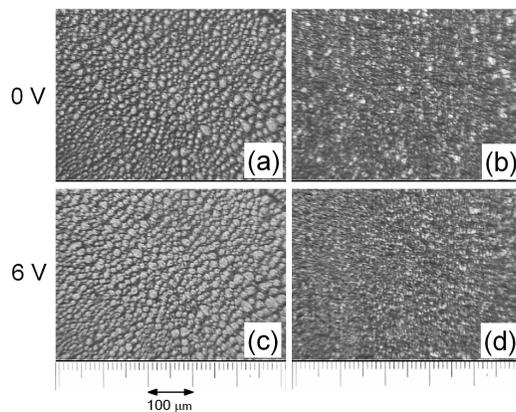
Figure 2. Optical polarizing microscopy images of the LC-polymer composite layer prepared in twisted cell. The pictures are taken when the cell is placed between two crossed polarizers: (b,d) the direction of the rubbed grooves coincide with one of the optical axes of the polarizers; (a,c) the cell is rotated at  $45^\circ$ . Applied voltage: 0 V (a,b); 6 V at frequency 25 Hz (c,d). The temperature of the sample was fixed at  $20^\circ\text{C}$ .
