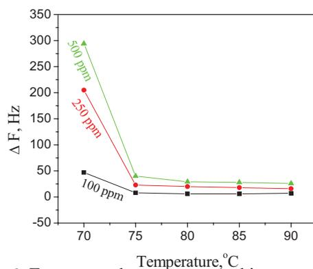
Figure 6: Frequency change versus etching temperature.
