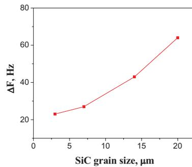
Figure 3: Change in QCM frequency as a function of abrasive grain size.
