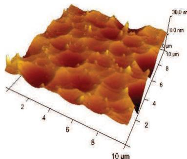
Figure 5: Surface of a quartz plate etched at 85°C. The average roughness is 3.71 nm.
