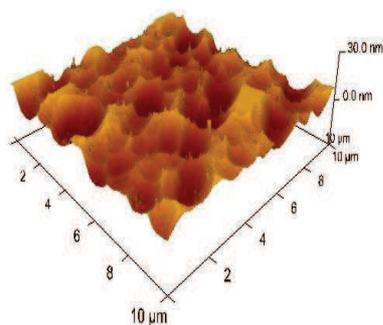
Figure 4: Surface of a quartz plate etched at 70°C. The average roughness is 4.51 nm.
