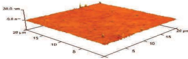
Figure 1: Polished surface. The average roughness ( $R_q$ ) is 0.612 nm.
