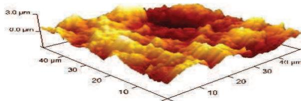
Figure 2: Surface of a plate processed with 20  $\mu\text{m}$  abrasive. The average roughness is 763 nm.
