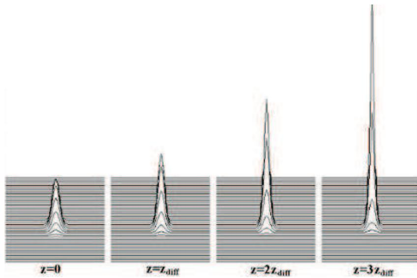
Figure 4: Propagation of an initial modulated optical pulse in medium with anomalous dispersion  $\beta = -0.5$  and coefficient of nonlinearity  $\gamma = 2.2$ . Plot of the side  $(x, t)$  projection.
