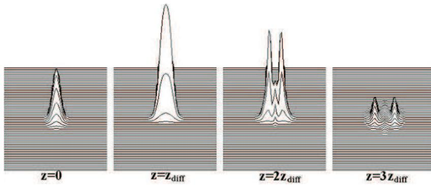
Figure 3: Nonlinear propagation of initially spatially modulated optical pulse in medium with normal dispersion  $\beta = 0.5$  and coefficient of nonlinearity  $\gamma = 2.2$ . Plot of the side  $(x, t)$  projection of the intensity  $|A(x, t)|^2$ .
