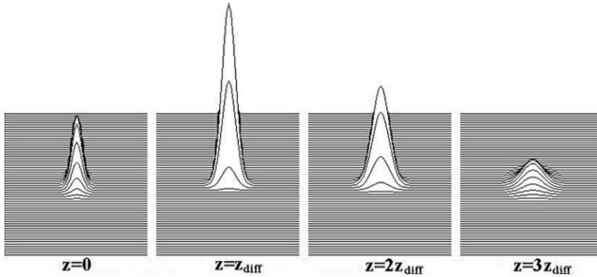
Figure 2: Plot of the side  $(x, t)$  projection of the intensity of the same pulse as in Figure 1. Now the propagation of this initially modulated optical pulse is in a solid medium with normal dispersion  $\beta = 0.5$ . The focus of the lens prevents the initial diffractive broadening. The dispersion leads to a significant increase of the time size of the pulse.
