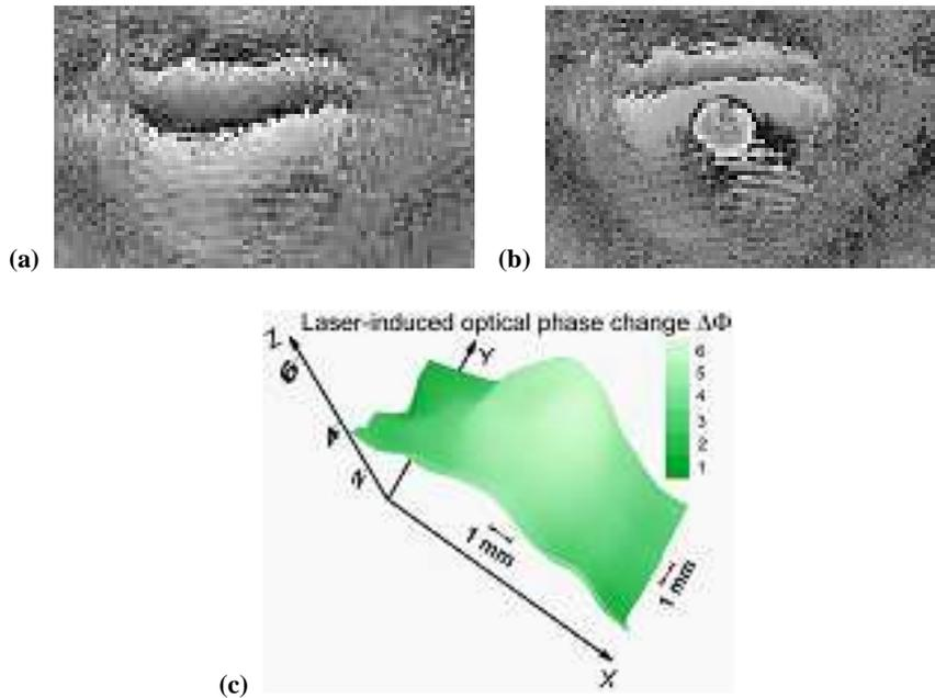
Figure 2: Optical phase profiles: (a) no pump; (b) pump present; (c) pump-induced optical phase change  $\Delta\Phi$  calculated from data in (a, b).
