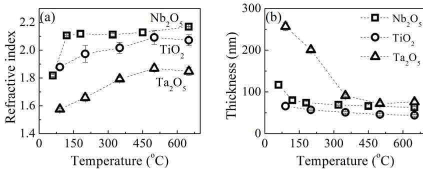
Figure 2: Refractive index at wavelength of 600 nm (a) and thickness (b) of  $Nb_2O_5$  (square),  $TiO_2$  (circle) and  $Ta_2O_5$  (triangle) films as a function of annealing temperature.
