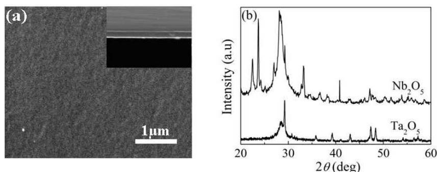
Figure 1: Surface and cross-sectional (inset) SEM images of  $\text{Ta}_2\text{O}_5$  film (a); XRD spectra of  $\text{Ta}_2\text{O}_5$  and  $\text{Nb}_2\text{O}_5$  annealed at 450°C for 30 min (b).
