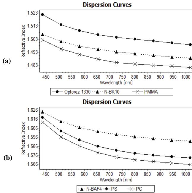
Figure 1: Dispersion curves calculated by means of OptiColor program of: (a) low; and (b) higher refractive OPs compared to glasses.
