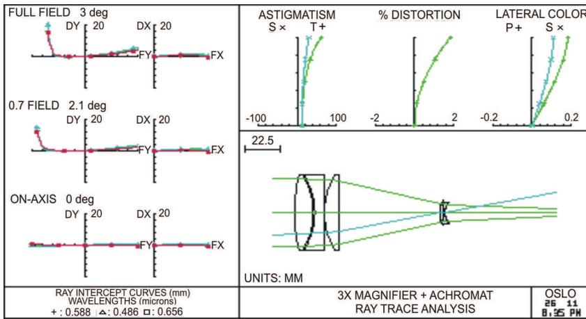
Figure 3: Optical scheme and geometrical aberrations of all-plastic magnifier and achromatic eyepiece.
