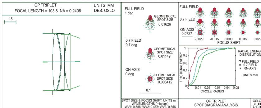
Figure 4: Optical scheme and spot diagram analysis of a hybrid triplet.
