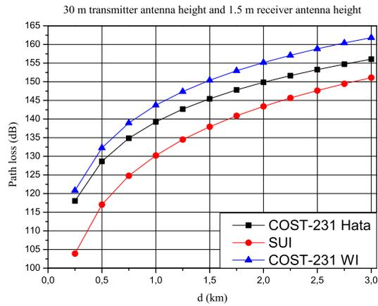
Figure 1: Path loss of the signal at the antenna height of the base station 30 m and height of the receiving antenna 1.5 m.
