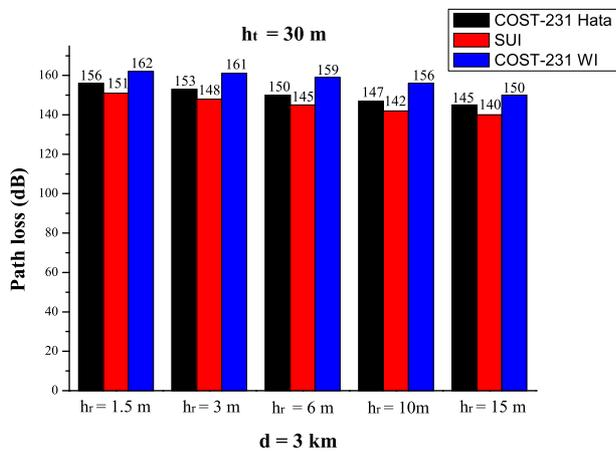
Figure 2: Results for PL at height of the transmitter antenna 30 m and receiving antenna height of 1.5 m to 15 m.
