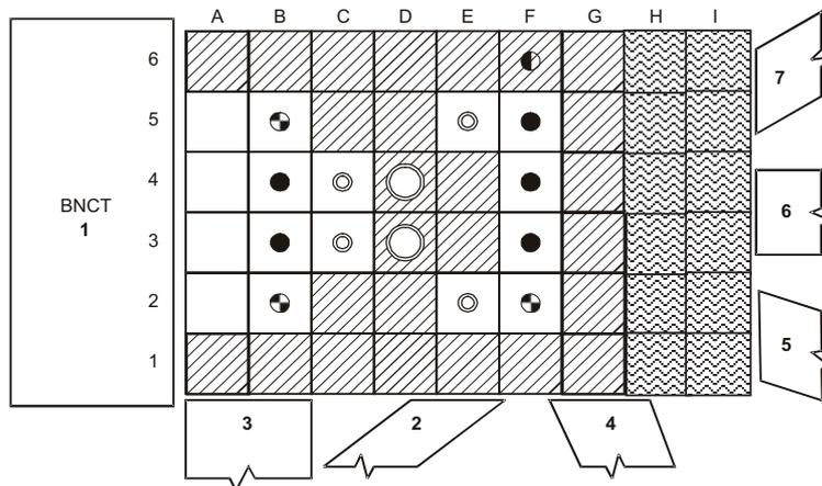
Figure 3. Initial core loading scheme of IRT-Sofia.
