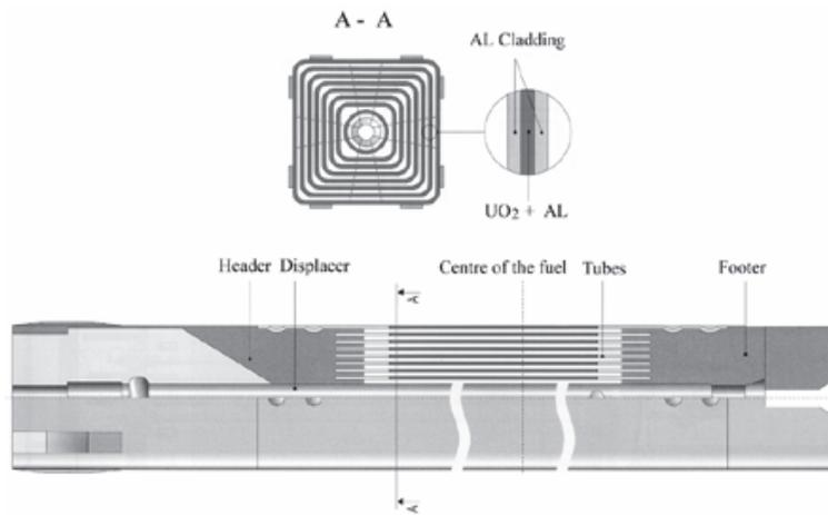
Figure 2. IRT-4M eight-tube assembly.
