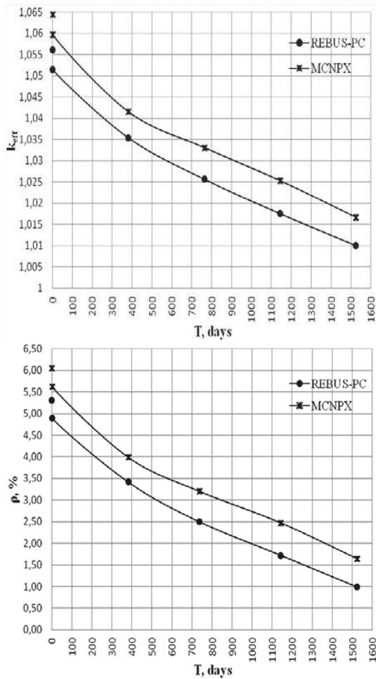
Figure 5. Changes with time in the effective neutron multiplication factor  $k_{eff}$  (left) and the excess reactivity (right) as a result from the calculations with REBUS-PC and MCNPX.
