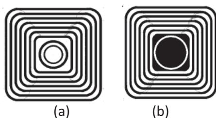
Figure 1. Transverse cross section view of IRT-4M tubular fuel assemblies: (a) eight-tube, (b) six tube.
