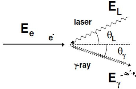
Figure 1. Geometry of the inverse Compton scattering of a laser photon with energy  $E_L$  incident at an angle  $\theta_L$  with respect to the axis of the relativistic electron beam. The photon is scattered at angle  $\theta_\gamma$  with respect to the electron beam.
