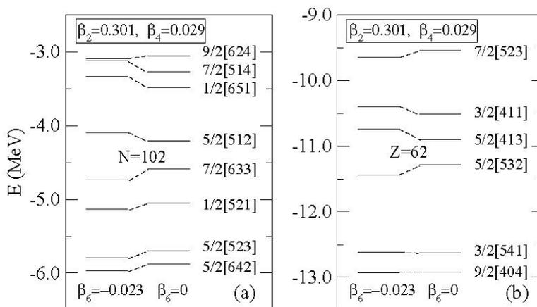
Figure 3. Neutron (left panel) and proton (right panel) single-particle energies with and without  $\beta_6$  deformation. Within each panel, the  $\beta_6 = 0$  levels are on the right.
