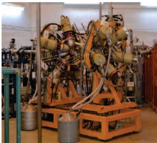
Figure 1. (Color online) The ROSPHERE array used in the mixed configuration with two types of detectors and with the plunger chamber.
