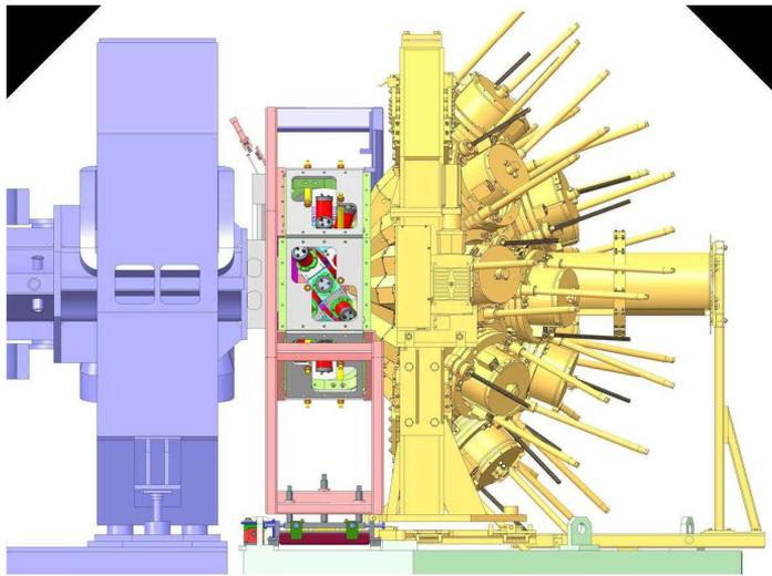
Figure 2. (Color online) Mechanical integration of FATIMA with VAMOS (in blue) and AGATA (in yellow). FATIMA  $\text{LaBr}_3\text{:Ce}$  detectors will be mounted on the EXOGAM structure, in between VAMOS and AGATA.
