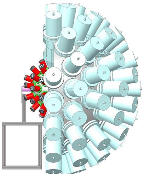
Figure 3. (Color online) Mechanical integration of FATIMA with Gammasphere.
