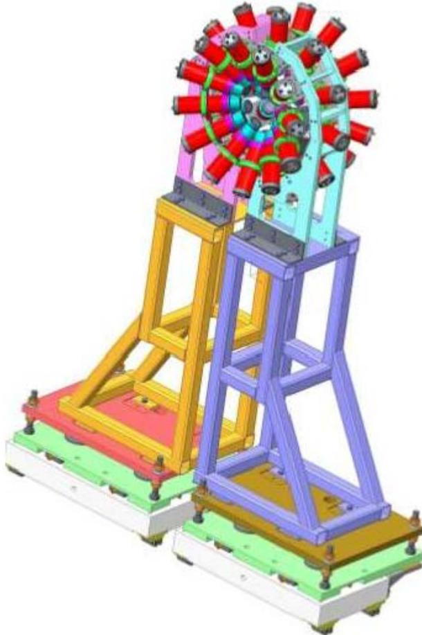
Figure 1. (Color online) A CAD image of the FATIMA array and support structure to be used at FAIR
