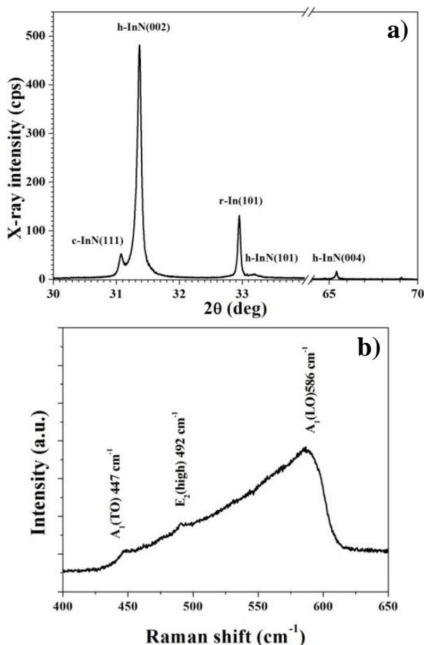
Figure 5. Typical (a) XRD and (b) Raman spectra of the InN nanowires (containing In-metal droplets on top).
