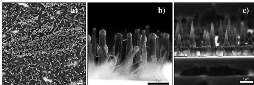
Figure 4. SEM micrographs of the as grown InN nanorods: (a) bird's-eye-view and (b) side view of the InN nanorods without indium desorption step at the end; (c) side view of the InN nanorods with 5 min indium desorption step at the end of the growth process.
