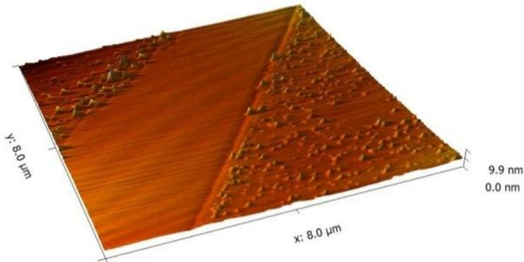
Figure 3. Sapphire substrate after annealing and nitridation: (a) SEM bird's-eye-view micrograph: triangular areas of different contrast can be distinguished; (b) AFM topography image on a surface including parts of both rough triangular (RMS = 0.6 nm) and the surrounding flat (RMS = 0.1 nm) areas.
