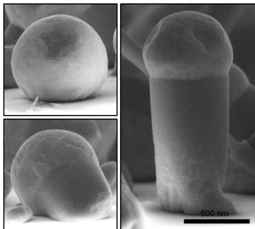
Figure 2. SEM micrographs of different stages of the InN nanowire growth: from droplet to the formation of the nanowire.
