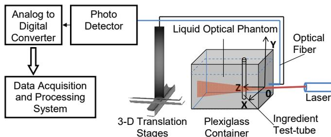
Figure 1. Experimental setup.
